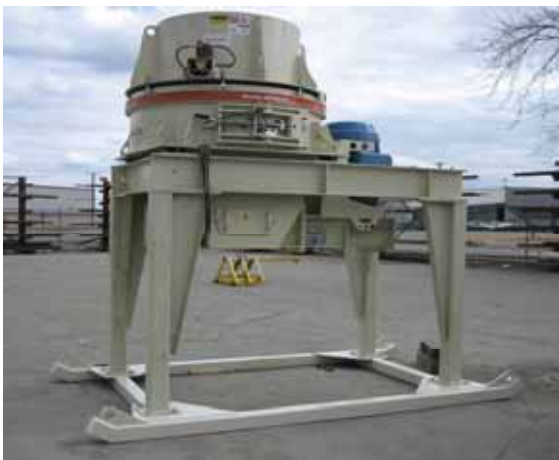
Components of the Barmac Vertical Shaft Impact (VSI) Crushing System
