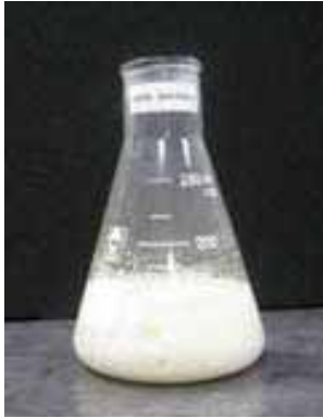
Marble Breaks down when exposed to the acid used in pool cleaning
