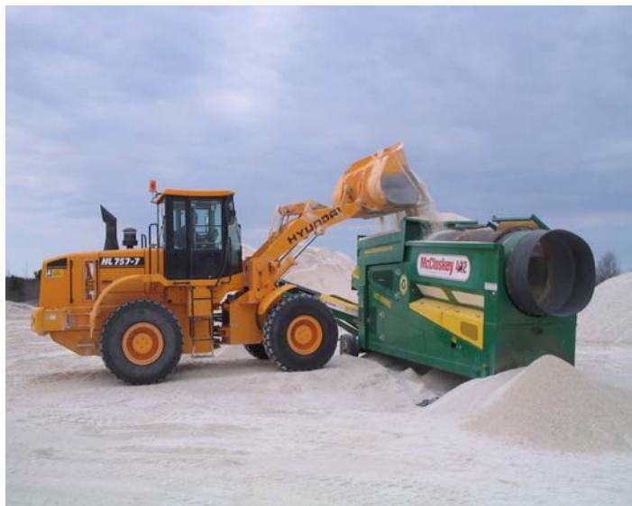
Sizing Material Prior to Feeding Quartz Processing Plant
